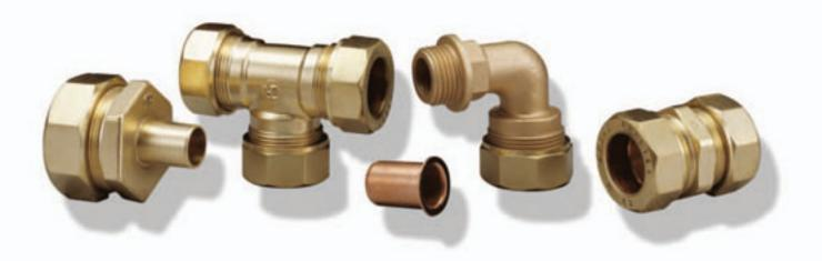
Manufactured to EN 1254-3 and EN 1254-4 and approved under the renowned WRc approval scheme, Prestex PL compression fittings are suitable for mechanically joining metric or imperial sized polyethylene by means of compressing a cone onto the tube which is internally supported by a stiffener.
